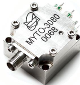
YIG-tuned oscillators MYTO maintain low phase noise signal even when output frequency varies more than one octave range. This can be reached with high-Q ferromagnetic yttrium-iron garnet resonators.
